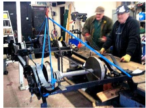
Wheels fitted and chassis re-assembled
