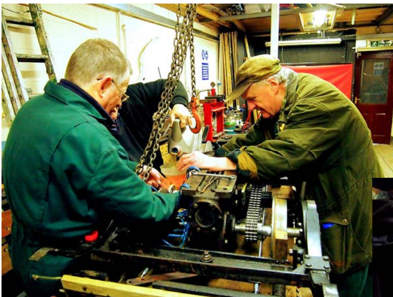
Little Tram gearbox filled with oil
